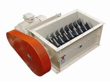
combs, along with hammer size and RPM allows some control over the finished particle size.
