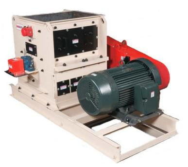
impact the material. In addition to the hammers, size reduction occurs through particle on particle contact and through contact with the breaker plate inside the grinding chamber. Because of their simplicity, the industrial hammer mill is easily adaptable to different sizes and mill designs. <u>Important to know:</u> Replaceable steel liner plates protect the mill's interior from wear caused by grinding abrasive materials.
