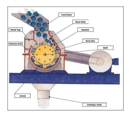
Hammer mills operate on the basic principle that most materials will crush, shatter or pulverize upon impact. This is accomplished by a simple four step process:
